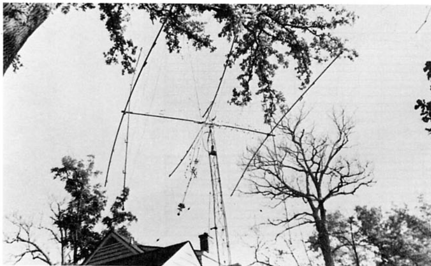
Fig. 11 — PV4-Quad on the author's former 34-foot tower.
